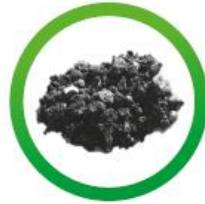
Reclaimed asphalt pavement (RAP)
