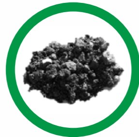
Reclaimed asphalt pavement (RAP)
